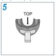
Check it is the right way up and that the notch is positioned at the top.
